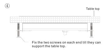
Above installation is for tabletop thickness witnin 5-40mm.
