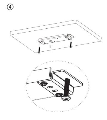
Above installation is for tabletop thickness within 5-35mm
