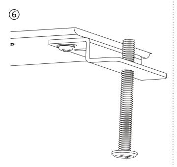
step 5 and 6 is for thickness within 35-50mm
